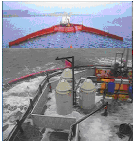
Figure 4: Wave Dragon Overtopping Device [14]
