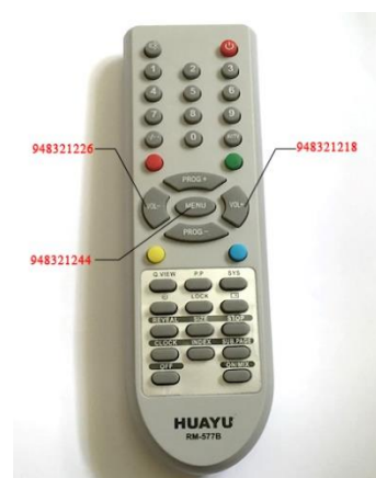
Figure 02: Codes generated for different buttons
