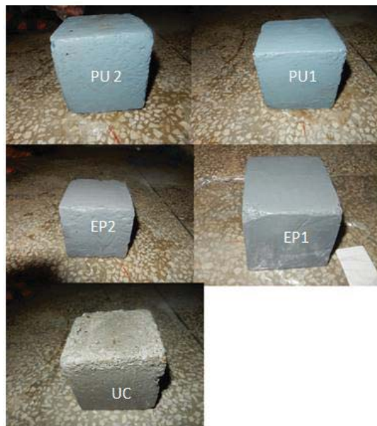
Figure 3. Samples after 120 hours in the acid bath
